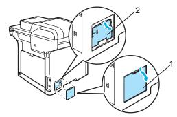
4 Unpack the DIMM and hold it by its edges.
